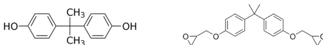
Figure 1. Chemical structure of bisphenol A (BPA, Left) and Bisphenol A diglycidyl ether (BADGE, right).
